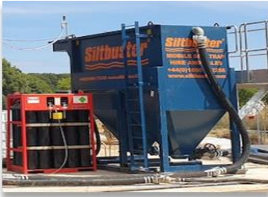
Graphic 3.11 Example of a Mobile Non-Active Waste-Water Treatment Plant Lighting
