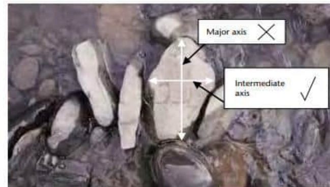
Figure E5 Illustration of correct use of the ‘intermediate axis’ for channel substrate assessments in RHS
